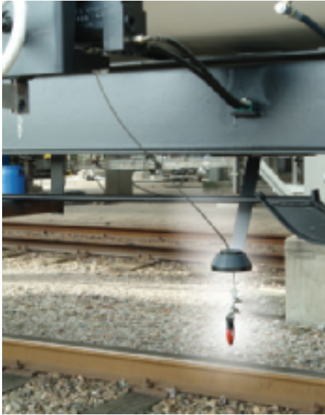
Figure 18 Connection ring and cable between the rail hook and the bottom valve of the RTC for closure of the bottom valve upon movement of the RTC
