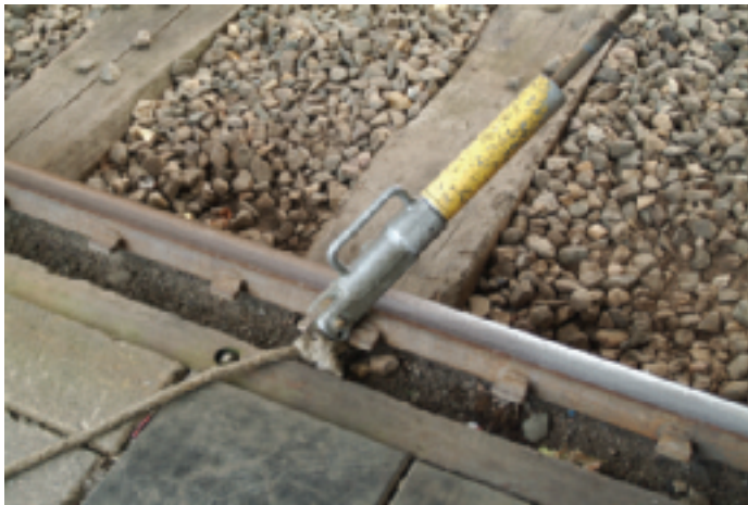
Figure 20 Rail hook, connected to the bottom valve cable, locked in the rails with manual release rope
