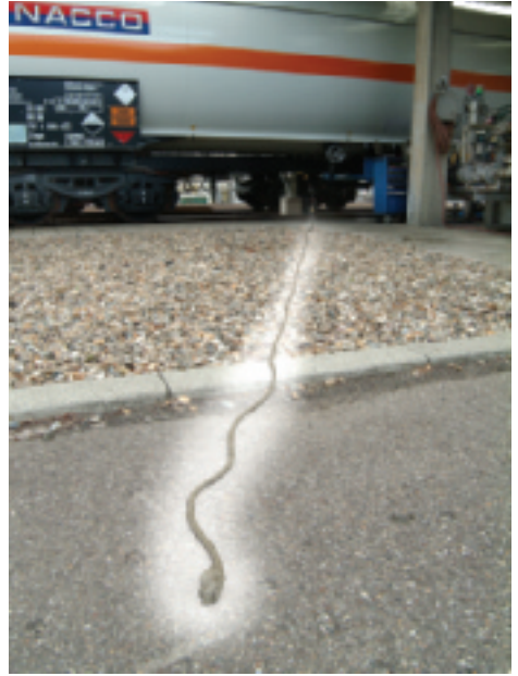
Figure 19 Release rope for distant closure of the bottom valve via the release of the rail hook in case of emergencies
