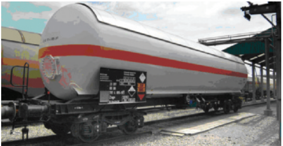
Figure 2 Typical example of an ammonia RTC showing the orange band, heat shield and identification plate
