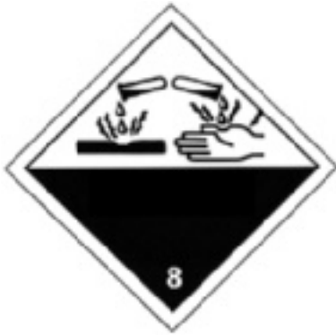
Figure 13 Danger label 8 Corrosive
