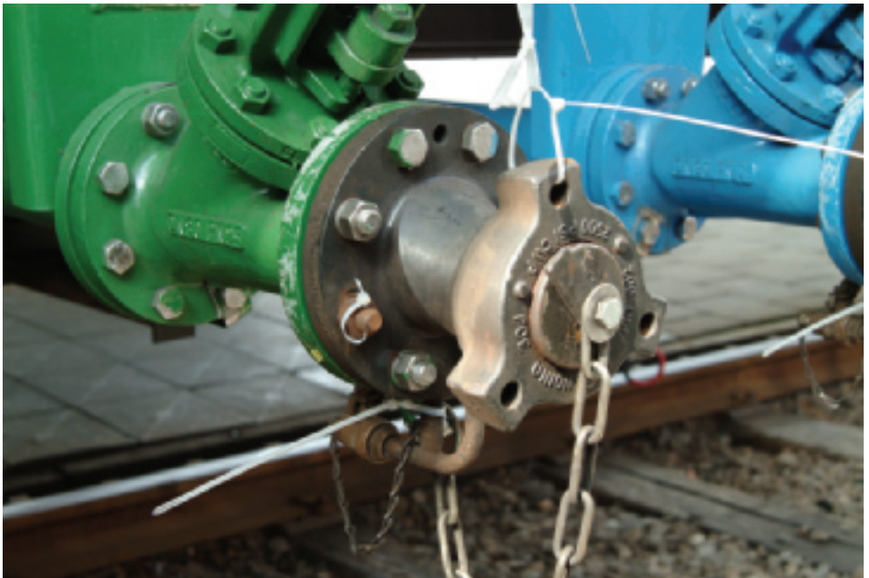
Figure 8 The screw-coupling with its protective cover ready for transport. Tie-raps are used to warn against unauthorised opening
