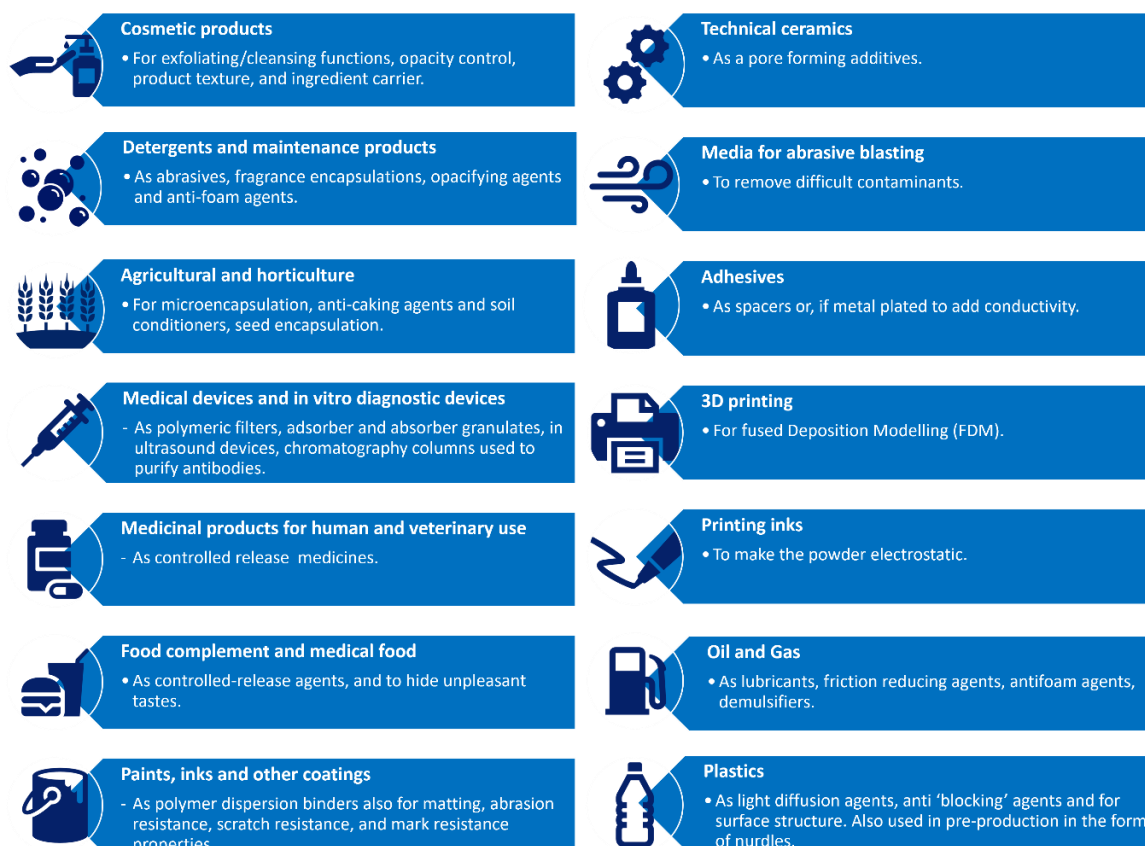
Figure 7-2 A selection of the main uses and functions of intentionally added microplastics
