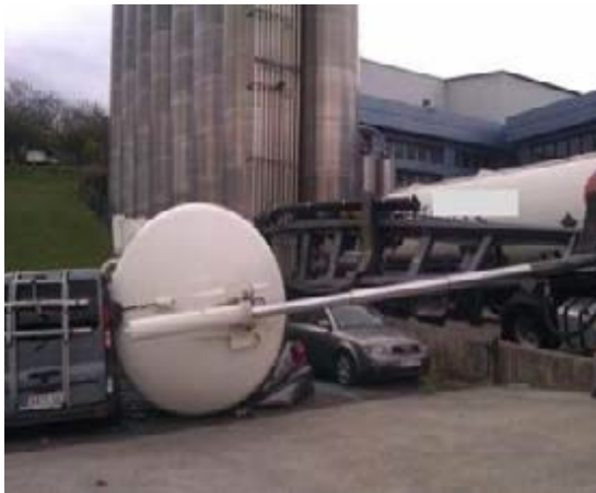
Trailer fell on parked cars during tipping
