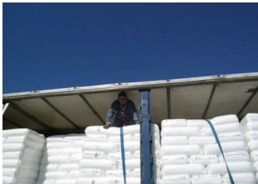
Driver climbing on top of pallets and increasing risk of falling
