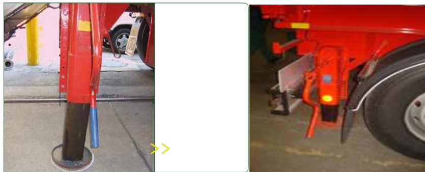
Bent stabilizing legs and should be changed
