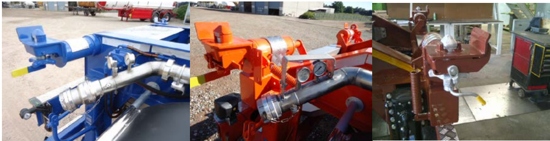
Twist locks with indicators and heel plates
