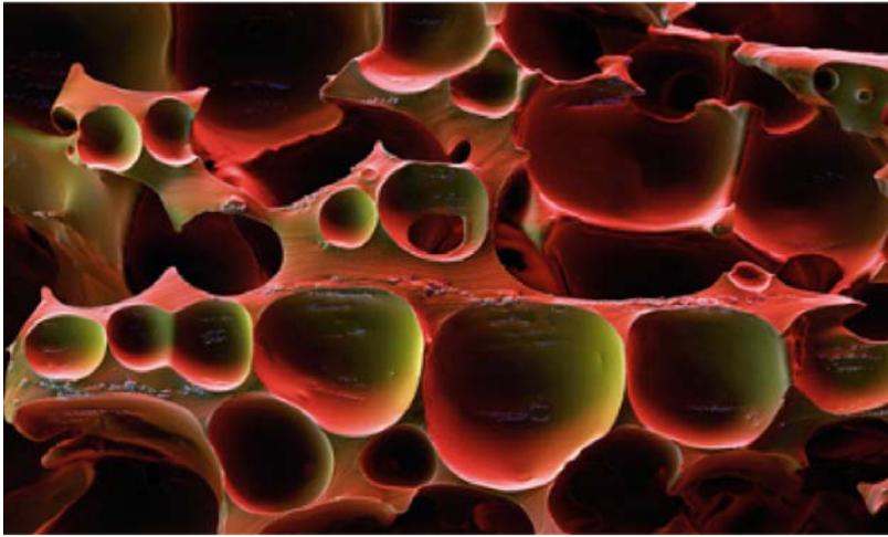
Polyurethane (PU) rigid foam systems are used in a number of cold and heat insulation applications. In addition to energy and cost savings, PU rigid foam offers architects freedom of design and additional living space due to slimmer construction options and as a result is used in house-building in a number of roof, wall and floor applications.
